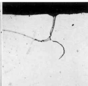
*Fig. 3* A 13 per cent rhodium-platinum wire after 1 hour at 1400°C in hydrogen with alumina insulators  $\times 320$
