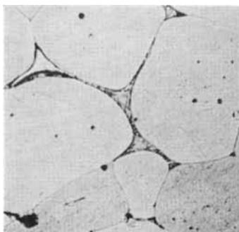
*Fig. 1* Platinum wire showing grain boundary embrittlement after 15 hours in hydrogen in an alumina tube  $\times 144$
