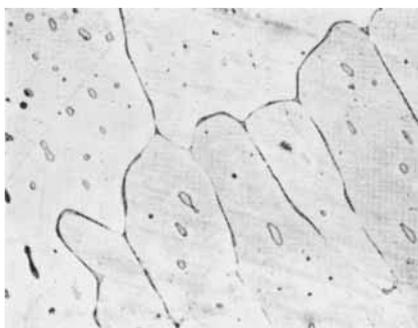
Fig. 4 The cast structure of a 0.3 per cent silicon-platinum alloy  $\times 320$
