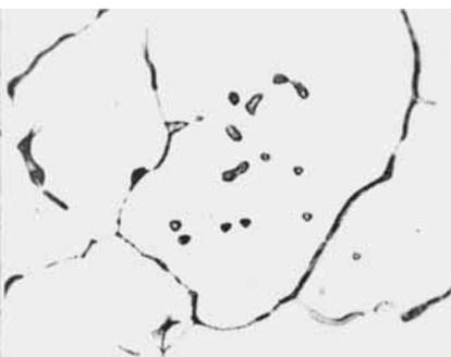
Fig. 5 The cast structure of a 0.6 per cent silicon-rhodium alloy  $\times 320$
