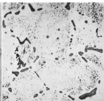
*Fig. 2* A 40 per cent iridium-rhodium wire embrittled after 96 hours at 1400°C in hydrogen in an alumina tube  $\times 320$
