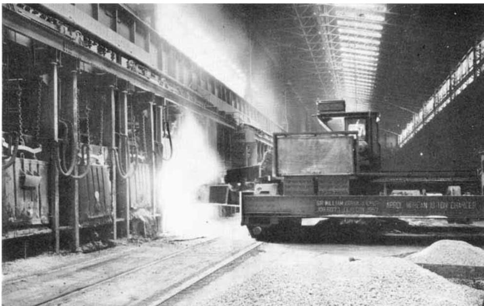
*Charging a box of iron ore to an open hearth furnace. The method of timed temperature measurements, in conjunction with rapid checks on the carbon content of the bath, makes it possible to decide on the exact moment when ore should be charged, so reducing the overall operating time*
