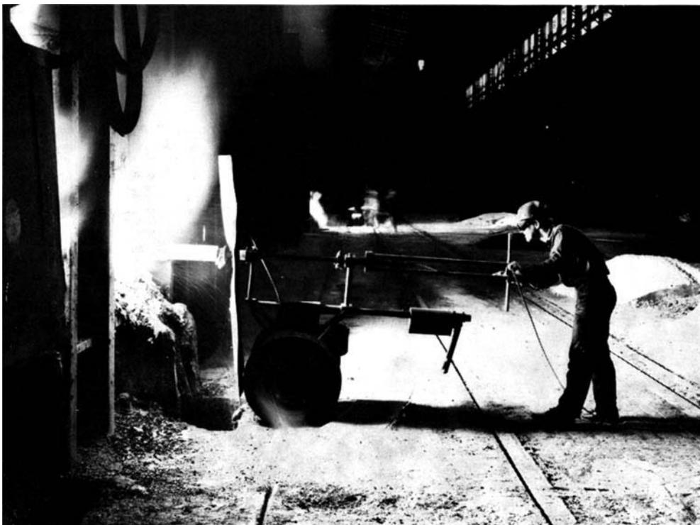
*Measuring the temperature of the charge with a platinum:rhodium-platinum thermocouple pyrometer in one of the 250-ton open hearth furnaces in the new melting shop at Colvilles' Ravenscraig works. Measurements made at fixed intervals of time are used to control the working of the charge and to increase the speed of reaction*
