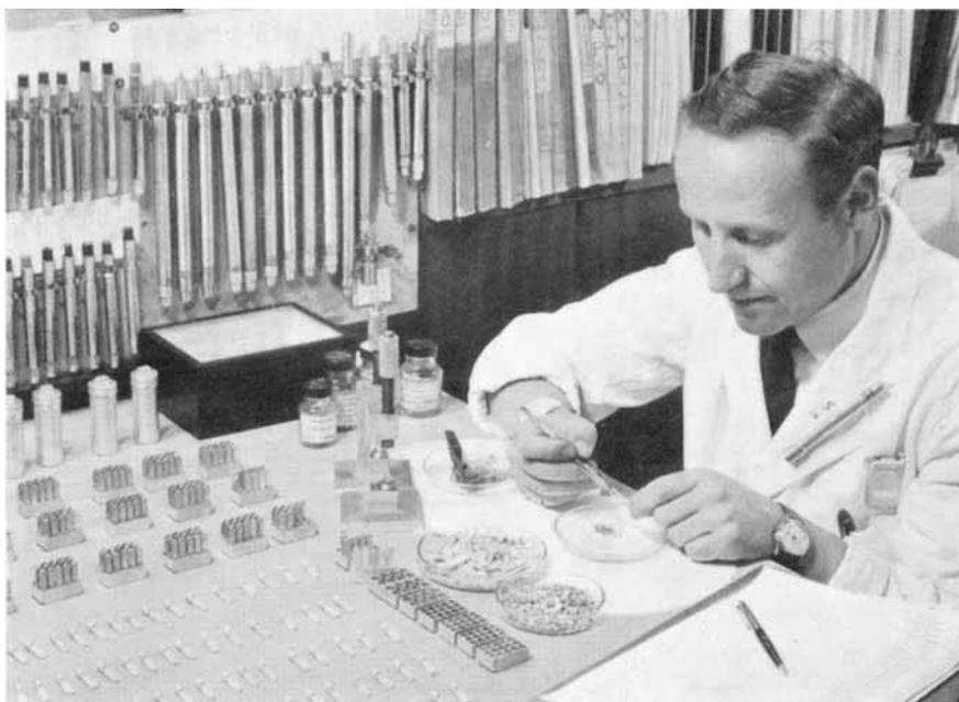
*The preparation of iridium-192 radiography sources. Inactive iridium cylinders are mounted in capsules in which they will be activated in a nuclear reactor*
