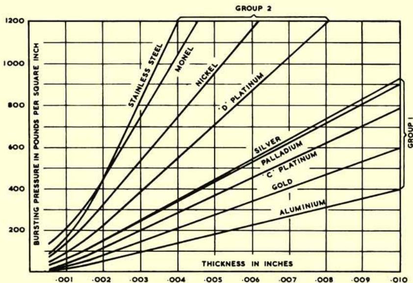
The relationship between pressure  $P$  and original thickness  $T$  for various disc materials in an orifice of one inch diameter ( $D$ ). For other orifice diameters the bursting pressure may be calculated from the formula  $DP/T=K$ , where  $K$  is a constant for a particular material.
