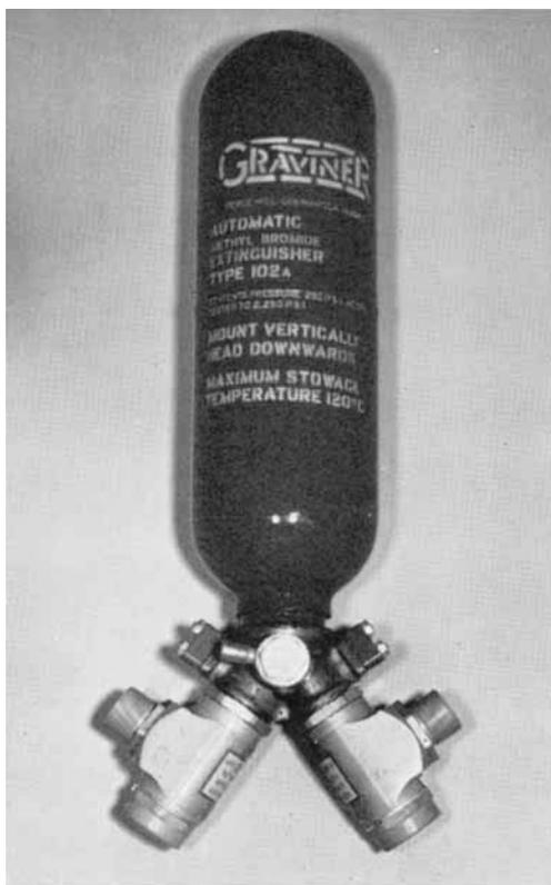
*In the Graviner fire extinguishing equipment used in jet aircraft a platinum bursting disc is fitted at the three-way junction to relieve internal pressure due to inadvertent overheating*
