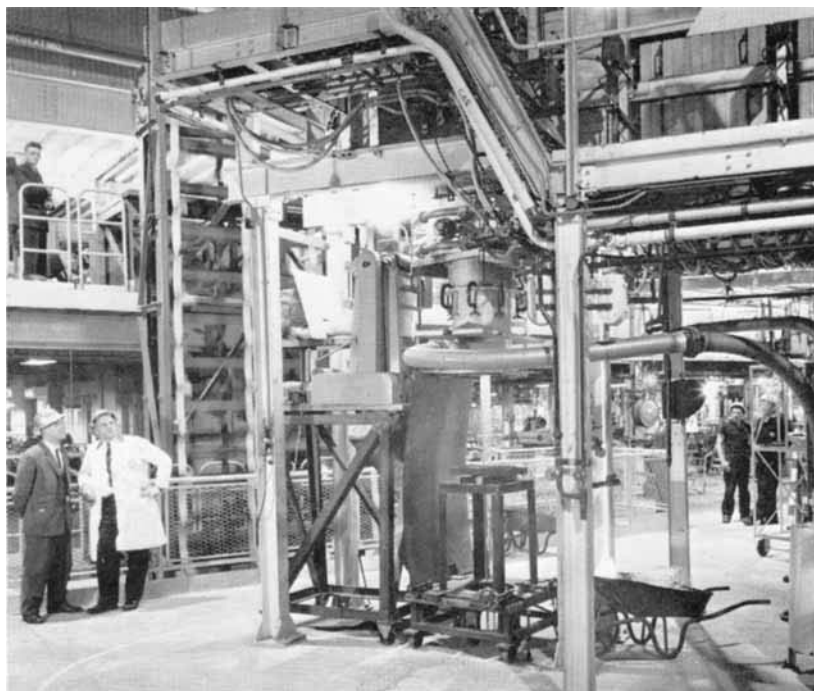
The new down-draw tubing machine at James A. Jobling & Company's Wear Glass Works. Pyrex tubing is produced by drawing molten glass over a platinum-clad mandrel.
