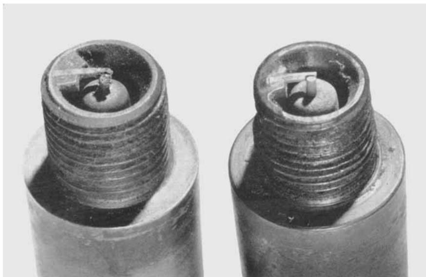
*On the left is a K.L.G. tungsten-platinum plug after 52 hours in a Bristol Centaurus engine. It already shows the onset of spark erosion from lead attack. The plug on the right is one of the new K.L.G. iridium plugs removed after 925 hours in the same engine. As can be seen, the plug was not cleaned or serviced before the photograph was taken.*
