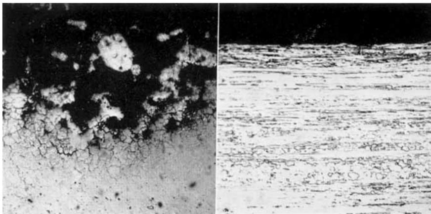
*Photomicrographs ( $\times 120$ ) of spark plug electrodes after 65 hours running in a single cylinder engine test by Bristol Siddeley Engines Ltd. The tungsten-platinum electrode (left) shows severe lead attack; the iridium electrode (right) is unattacked.*
