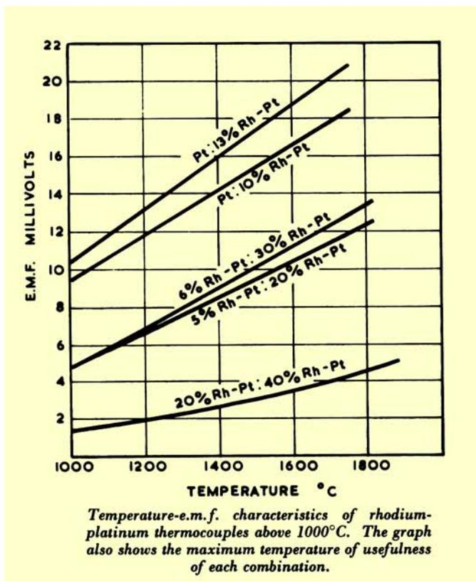
per cent rhodium have a melting point of approximately 1820°C, so that couples employing one of these as the negative limb can be used to measure temperatures up to 1800°C for a short time. The 20:40 combination, although capable of measuring up to as high as 1850°C for short periods, gives an appreciably lower e.m.f. The relative e.m.f. characteristics of these thermocouples above 1000°C, and their maximum temperatures of use, are shown in the graph.
