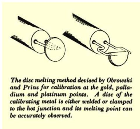
*The disc melting method devised by Obrowski and Prinz for calibration at the gold, palladium and platinum points. A disc of the calibrating metal is either welded or clamped to the hot junction and its melting point can be accurately observed.*
