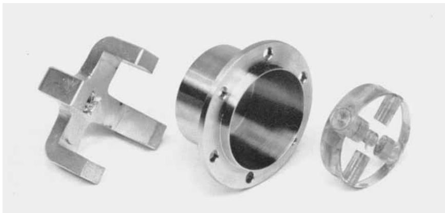
Component parts of the magnet drive showing the four-pole cobalt-steel claw magnet, the tantalum separating cup and the Platinax II magnet assembly containing four magnets backed by pieces of soft iron to increase their effective length.
