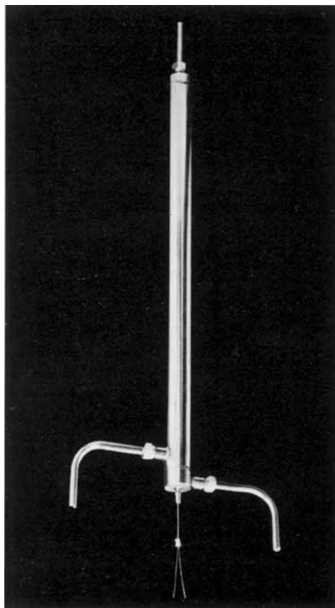
Fig. 2 A Johnson Matthey silver-palladium alloy diffusion cell, showing the ultra-pure hydrogen outlet uppermost
