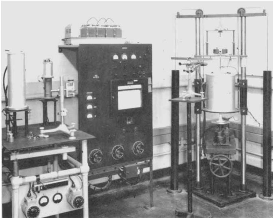
*The laboratory equipment for viscosity determination. On the right is the rotating cylinder apparatus; on the left the furnace for determining the viscosity of glass fibres*
