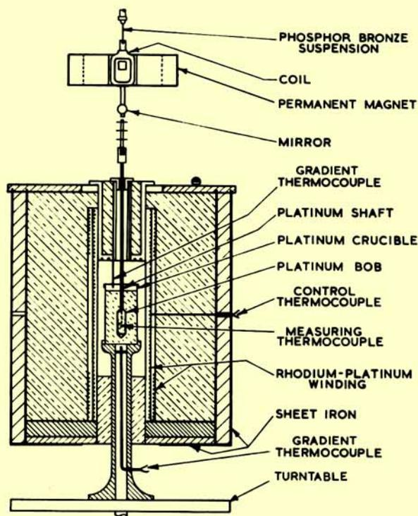
*Constructional diagram of the high temperature furnace designed by the National Bureau of Standards for determining the viscosity of molten glass*
