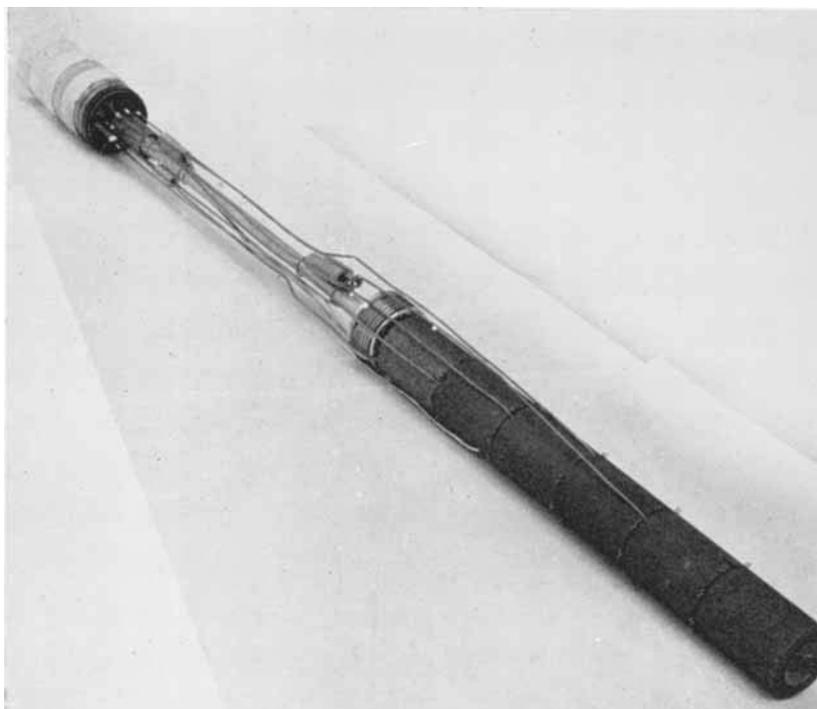
*Part of a test capsule used in an irradiation experiment in the Dragon Reactor. Fuel is contained in the graphite cylinders and the temperature distribution along the capsule is measured by the metal-clad molybdenum-platinum thermocouples which may be seen protruding through the gaps between the cylinders*
