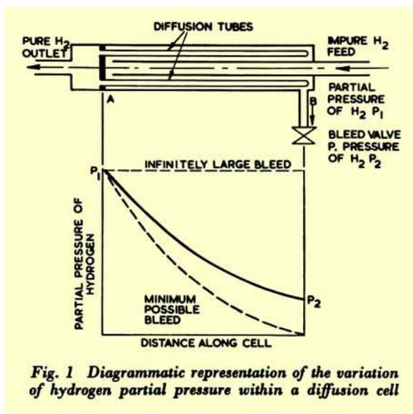
Fig. 1 Diagrammatic representation of the variation of hydrogen partial pressure within a diffusion cell
