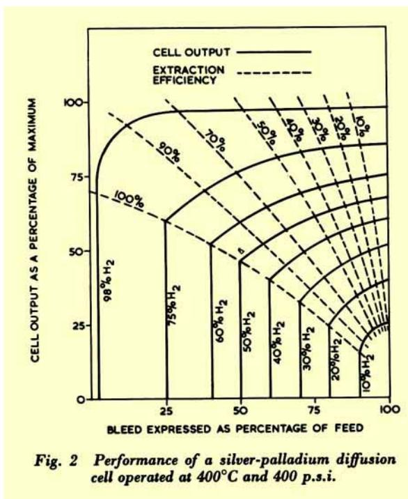
Fig. 2 Performance of a silver-palladium diffusion cell operated at 400°C and 400 p.s.i.
