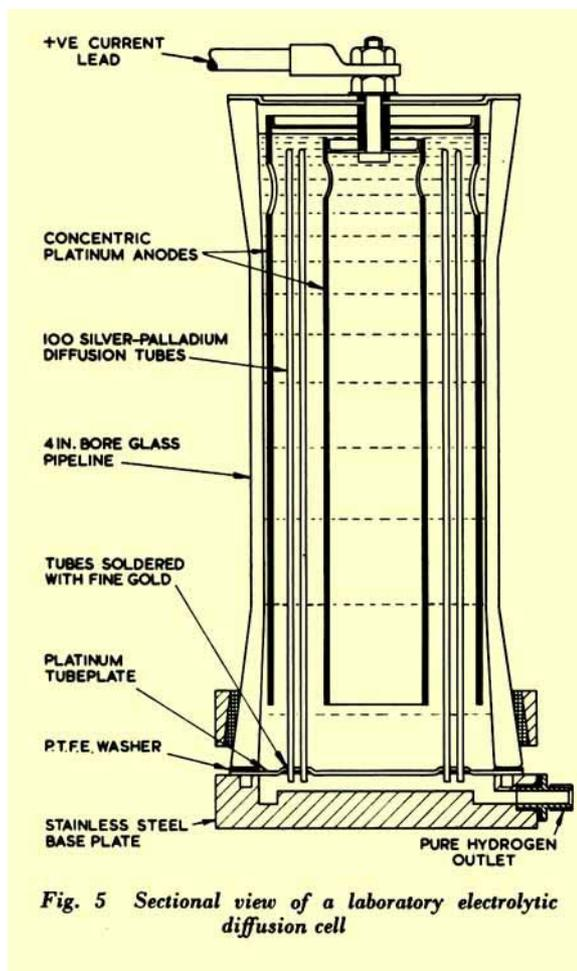
but the total demand does not justify a high capital outlay. Electrolytic cells of the type described can work against outlet pressures of 400 p.s.i. and are conveniently used for supplying laboratory sintering furnaces with pure hydrogen, for gas chromatography and for hydrogenation experiments in organic chemistry.
