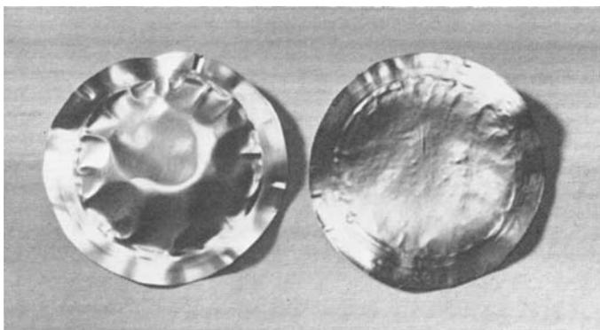
Fig. 3 Appearance of a pure palladium electrode (left) and a silver-palladium electrode after five cycles of charge and discharge
