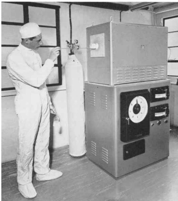
The furnace is 37 inches long and has a bore of  $2\frac{1}{2}$  inches. The axis of the bore of the furnace is 63 inches above floor level.
