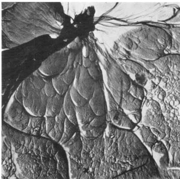
*The platinum metals will be used in most fuel cell designs in diffusion-type electrodes in the form of high surface area "blacks" in order to achieve the highest possible activity per gram of metal. This electronphotomicrograph of a platinum black electrode surface of high catalytic activity demonstrates the very complex structure of platinum black itself (x 20,000)*
