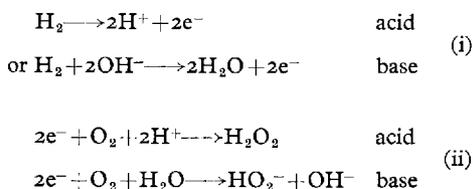
The high values of  $i_0$  are associated with the low heat of chemisorption of hydrogen and oxygen on platinum metals.
