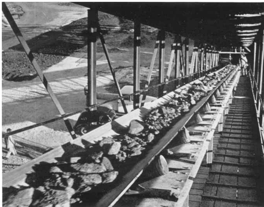
Platinum ore being transported by conveyor belt up to the sorting station in the reduction plant at Rustenburg
