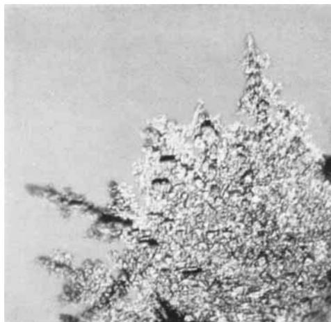
*Large platinum crystals detached from a dismantled platinum heated furnace after long service at high temperatures. These formed adjacent to the heating elements ( $\times 12$ )*
