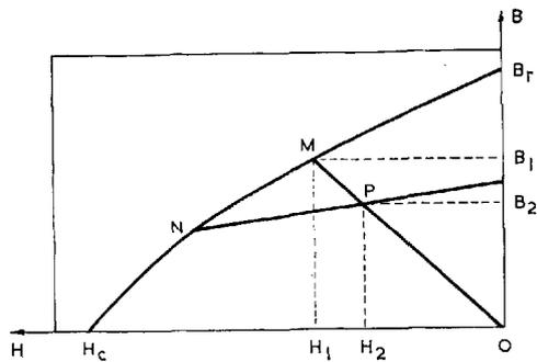
Fig. 3 The working point of a magnet subjected to a demagnetising field follows the curve from M to N. When the field is removed, a partial recovery is made and the working point moves along a recoil line to the position P. The performance of the magnet undergoes a corresponding change
