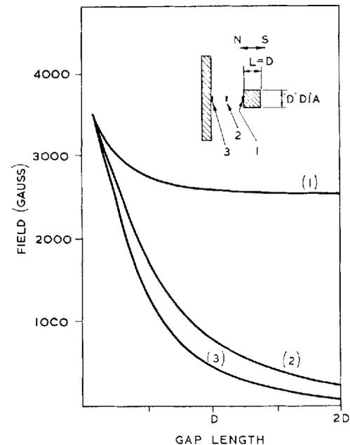
Fig. 8 An improvement on "open-circuit" working is obtained by placing the magnet near an iron plate. For a magnet with an  $L/D$  ratio of 1, this results in a 40 per cent increase in the maximum measured field
