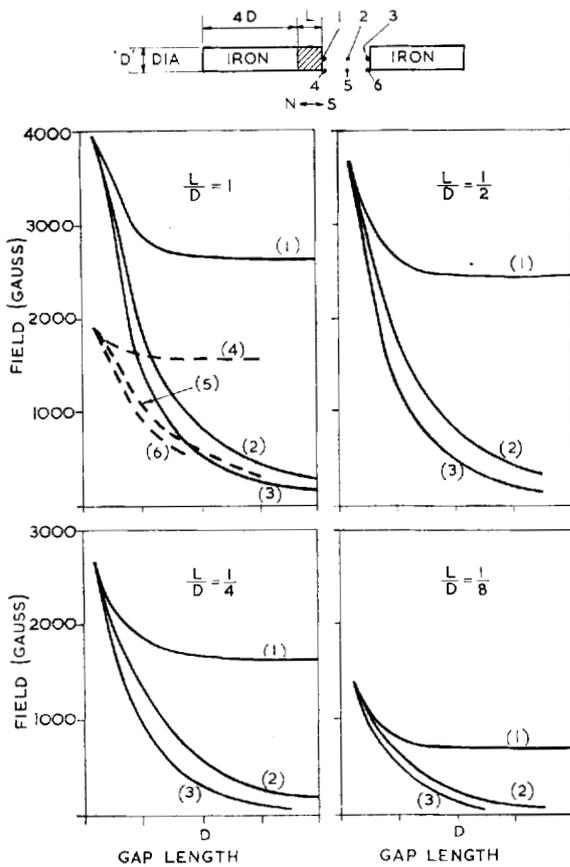
Fig. 9 Improved performance is obtained by extending the magnetic circuit with iron cylinders. The increase in field over "open-circuit" figures ranges from approximately 50 per cent for the longest magnet ( $L/D = 1$ ) to nearly 250 per cent for the shortest ( $L/D = 1/8$ ). The axial fields were measured at positions 1, 2 and 3, and the edge fields at positions 4, 5 and 6
