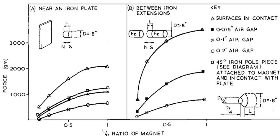
Fig. 11 Forces produced by Platinax II magnets vary with magnet geometry and the type of circuit in use. Examples of two basic circuits are given, showing the forces produced under a variety of conditions
