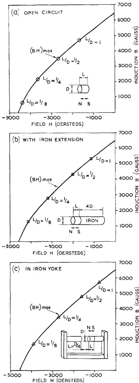
Fig. 2 A magnet's performance is governed by its shape and the type of circuit in which it works. Measurement of the working points of Platinax II magnet systems shows that (a) high performance is obtained from short, open-circuit magnets. Greater economy is achieved by (b) adding a short iron extension and by (c) placing the magnet in an iron yoke
