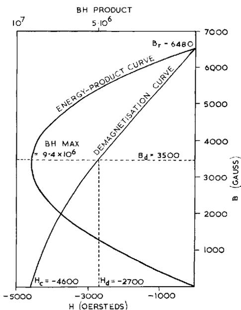
The working points of four cylindrical magnets are shown in Fig. 2 on the demagnetisation curve for Platinax II. Each magnet was measured in three separate circuits, covering a wide range of self-demagnetising conditions.
