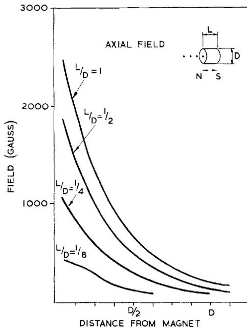
Fig. 6 The axial fields produced by "open-circuit" Platinax magnets vary with distance from the magnet. The effect of the increased self-demagnetisation of shorter magnets is illustrated by the lower fields they produce
