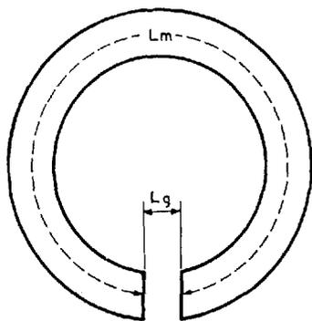
Fig. 5 A ring magnet with a short air gap
