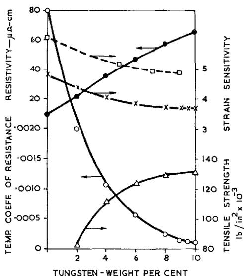
*Electrical and mechanical properties of tungsten-platinum alloys. All specimens were in the annealed condition except that represented by the broken line, which was in the hard drawn state.*
