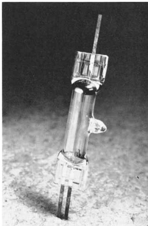
*The quartz arc tube of a 125 watt type MBU mercury vapour lamp by Osram (G.E.C.) Limited. The reflecting surfaces at each end of the tube are thin films of gold-platinum alloy serving as infra-red reflectors and so eliminating local cold spots in the region of the electrodes*
