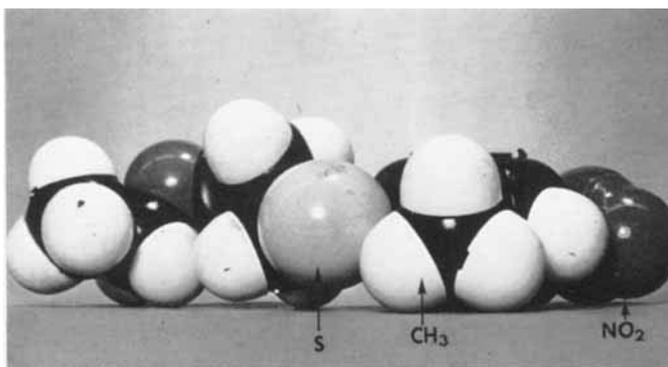
Fig. 7 Ethyl (2-methyl-4-nitrophenyl) mercaptopropionate; the methyl group inhibits contact between the sulphur atom and the catalyst surface and hydrogenation of the nitro-group proceeds, although slowly. (This model is somewhat idealised for photographic purposes. The sulphur atom is actually closer to the surface and the 2-methyl group restricts rotation to prevent firm attachment of the sulphur to the catalyst)
