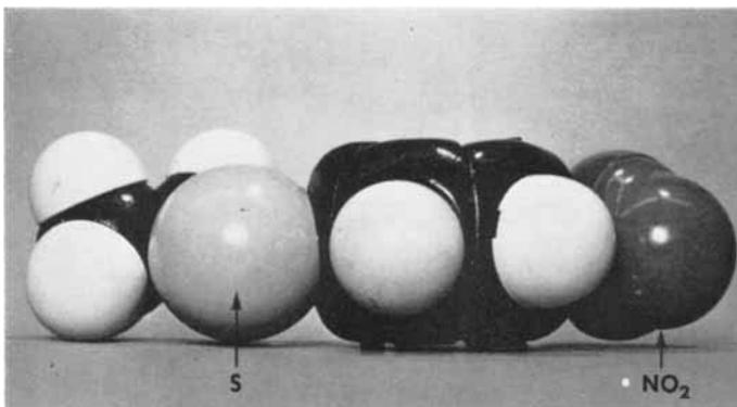
Fig. 6 Ethyl 4-nitrophenyl sulphide: in this molecule the sulphur atom can easily touch the catalyst surface, suggesting that poisoning will occur
