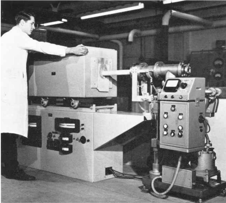
*The high temperature platinum-wound vacuum furnace installed in the Johnson Matthey Research Laboratories*
