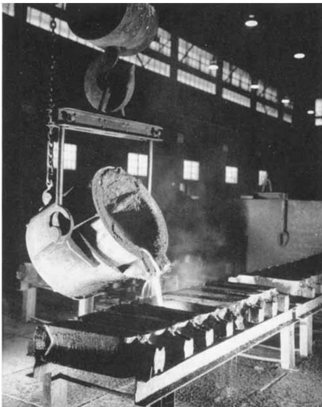
*An early stage in the process in the Johnson Matthey smelting plant. Nickel matte, carrying with it the platinum metals, is cast into pigs*
