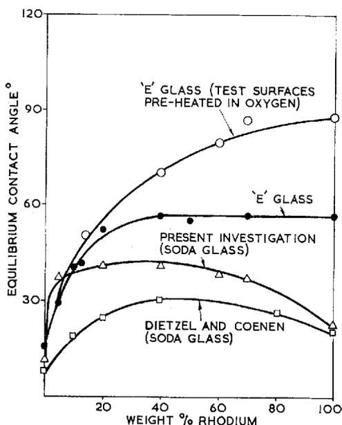
Fig. 3 Contact angles assumed by droplets of soda glass and "E" glass on rhodium-platinum alloys. Alloys having a high rhodium content oxidise when heated in air and this increases considerably the equilibrium contact angle
