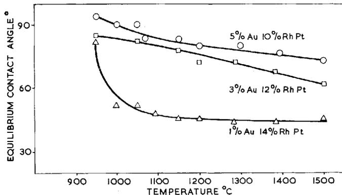
Fig. 7 Effect of temperature on the equilibrium contact angle of "E" glass melted on some representative ternary alloys. The temperature dependence decreases rapidly with increasing gold content. With 5 per cent of gold present the contact angle still exceeds 70° at 1500°C
