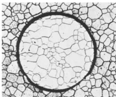
Fig. 8 Plan view of the etched surface left behind after removal of a glass bead from a 5 per cent gold-10 per cent rhodium-platinum test piece ( $\times 30$ )
