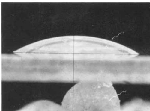
Fig. 11 Droplet of "E" glass in equilibrium with the surface of a 10 per cent rhodium-platinum alloy heated in air at 1200°C ( $\times 20$ )
