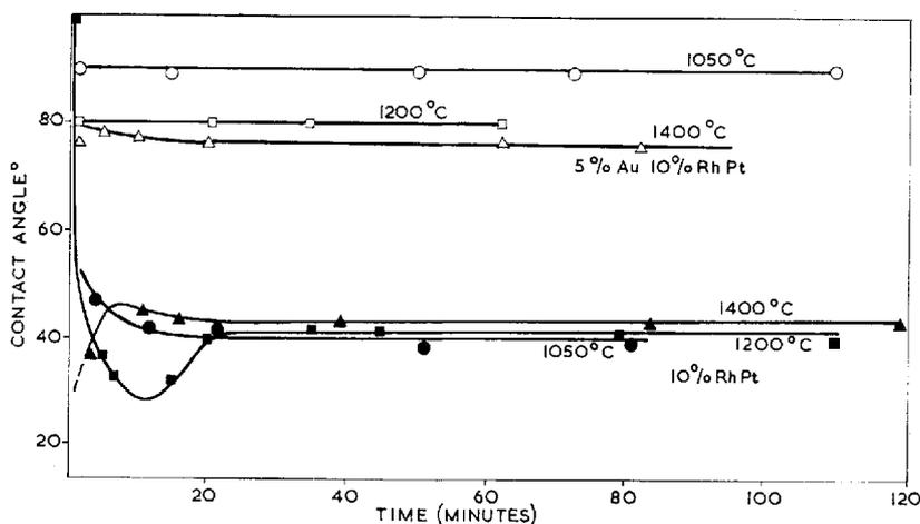
Fig. 1 Curves showing the effect of time on the contact angle between "E" glass and two platinum alloys maintained in air at constant temperature
