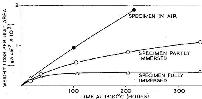
Fig. 9 Curves showing the loss of weight of test plates of the 5 per cent gold-10 per cent rhodium-85 per cent platinum alloy fully and partly immersed in molten "E" glass at 1300°C. Specimens immersed in glass decreased in weight less rapidly than those hung in air at the same temperature
