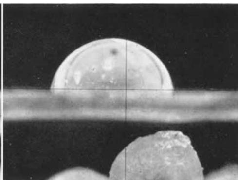
Fig. 12 The high contact angle assumed by a droplet of "E" glass melted in air at 1200°C on the surface of a 10 per cent rhodium-platinum alloy containing 5 per cent of gold ( $\times 20$ )
