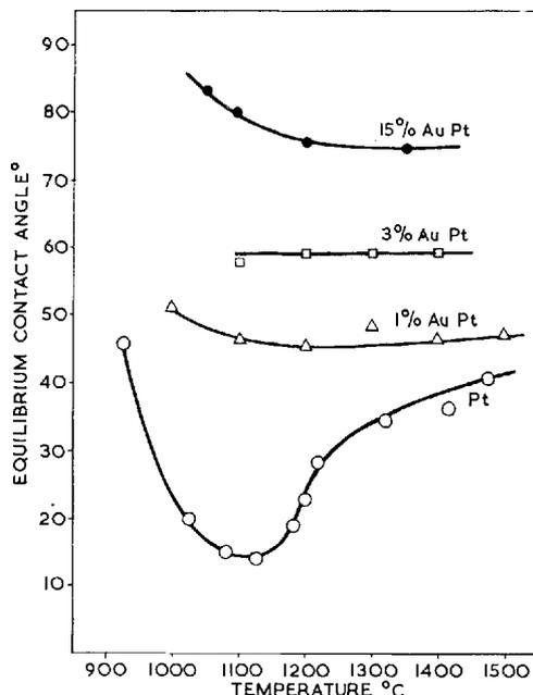
Fig. 4 Effect of temperature on the equilibrium contact angle of "E" glass on gold-platinum alloys heated in air. The addition of even 1 per cent of gold to platinum increases considerably the contact angle assumed by borosilicate glass
