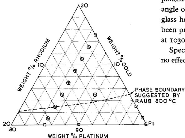
Fig. 5 Diagram showing the compositions of the gold-rhodium-platinum alloys studied in relation to the position of the phase boundary at 800°C suggested by Raub
