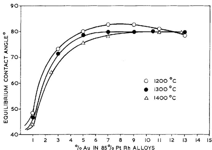
Fig. 6 Effect of gold on the equilibrium contact angle of "E" glass on ternary alloys containing 85 per cent of platinum
