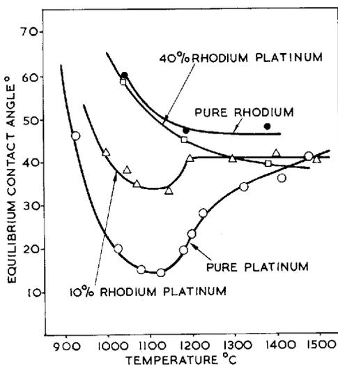
Fig. 2 The effect of temperature on the equilibrium contact angle of "E" glass on rhodium-platinum alloys heated in air. Although rhodium increases the contact angle considerably at lower temperatures, the increase becomes marginal even with very high rhodium contents above 1200°C
